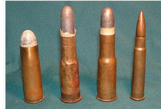
(From Left to Right): A .577 Snider cartridge, a Zulu War-era rolled-brass-foil .577/450 Martini-Henry Cartridge, a later drawn-brass .577/450 Martini-Henry cartridge, and a .303 British Mk VII SAA Ball cartridge.
