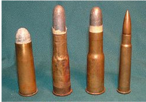
(From Left to Right): A .577 Snider cartridge, a Zulu War-era rolled brass foil .577/450 Martini-Henry Cartridge, a later drawn brass .577/450 Martini-Henry cartridge, and a .303 British Mk VII SAA Ball cartridge
